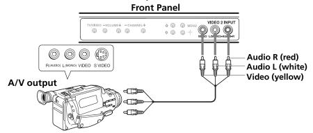
□ For better picture quality, use S VIDEO (located on the rear panel), instead of the yellow video cable. S VIDEO does not provide sound, so you still must connect the audio cables.
